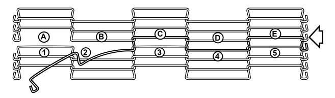
2. If you are installing a new belt, you are finished splicing.
